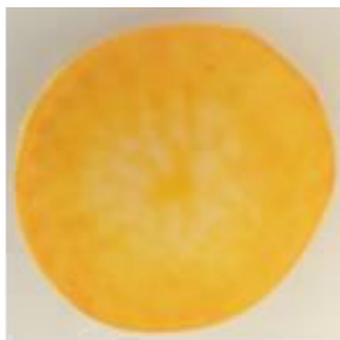
**Figure 2.** The polymer membrane with 20 wt.% *N,N'*-bis(salicylidene)ethylenediamine before the sorption process.
