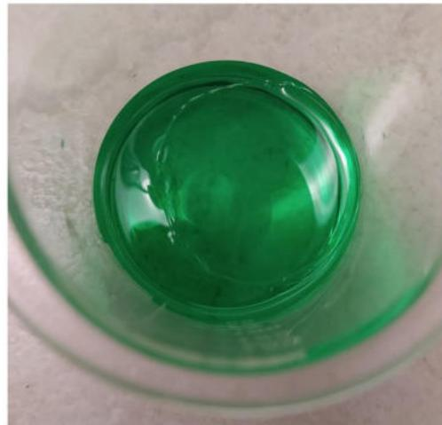
**Figure 5.** Polymer film immersed in nitric(V) acid solution.
