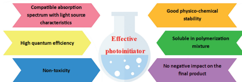
Fig. 2 Sample requirements for an effective photoinitiator.
