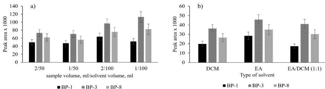
**Figure 2.** Optimization of MEPS method, sample spiked concentration  $100 \mu\text{g L}^{-1}$ , (a) effect of sample volume (1, 2 mL) and eluent volume (50, 100  $\mu\text{L}$ ) (EA/DCM, 1:1,  $v/v$ ); (b) selection of eluent (sample volume 1 mL, eluent volume 100  $\mu\text{L}$ ).
