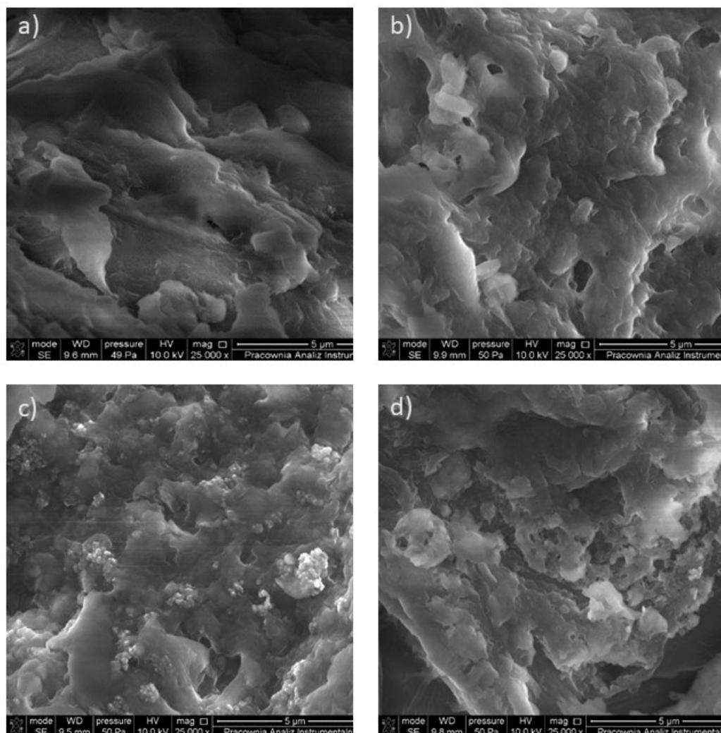
**Figure 3.** SEM images of (a) walnut shells; (b) walnut shells after adsorption of analytes; (c) peanut shells; (d) peanut shells after adsorption of analytes.
