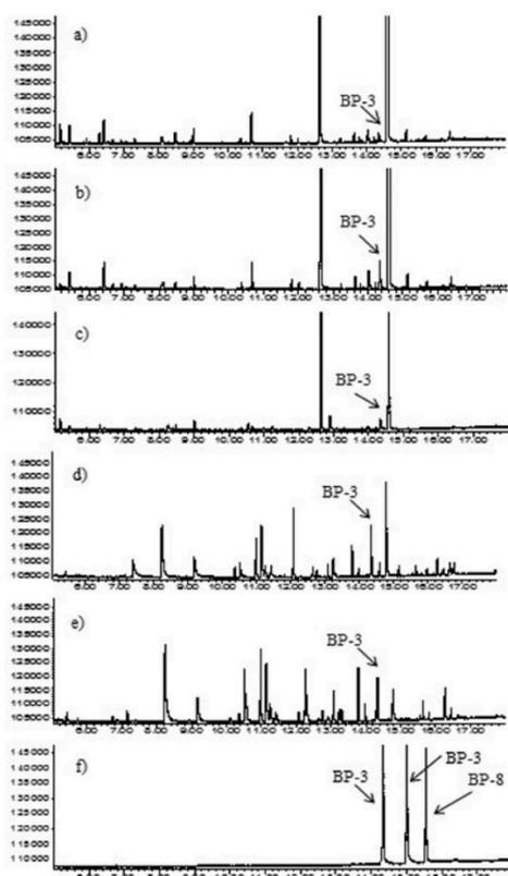
**Figure 1.** Chromatograms of (a) hair mask sample—SPE method; (b) hair mask sample with addition of BP-3 standard—SPE method; (c) hair mask sample—MEPS method; (d) shampoo sample—SPE method; (e) shampoo sample—MEPS method; (f) standard solution of BPs at concentration of 50  $\mu\text{g mL}^{-1}$ .
