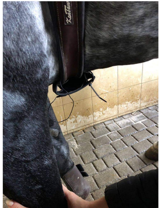
Fig. 1. The device Seaver girth sleeve on the horse girth. The cable is going to the heart rate electrode under the saddle, placed behind the withers on the left side of the horse, right where the saddle comes in contact with the horse's back (more details in Seaver manual – www.seaverhorse.com ).
