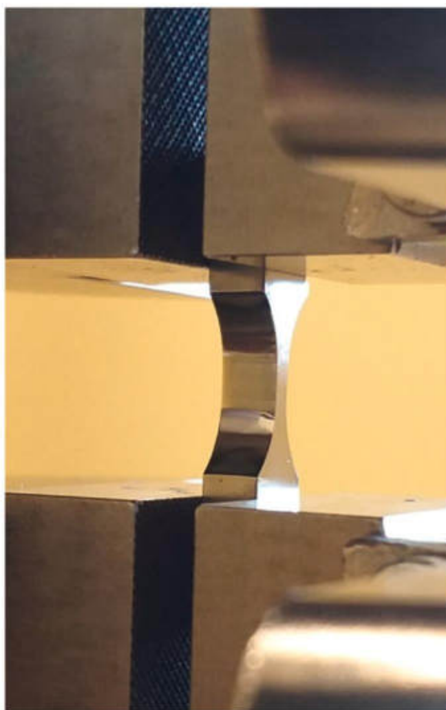
Fig. 2. Polished specimen mounted in the grips of the testing machine.
