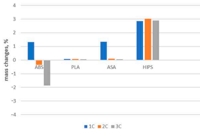
Figure 7. Changes in mass of sample after successive cycles.
